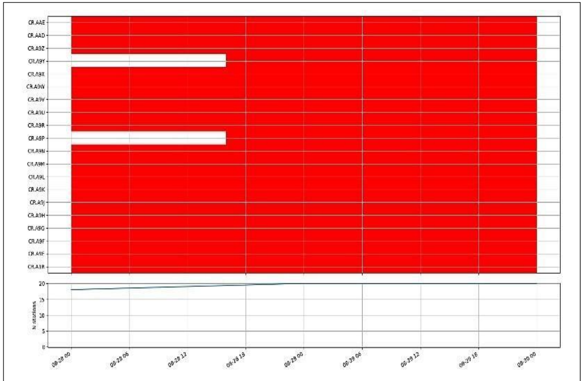
Figure 6.4: Data availability plot of seismic stations acquired from the tailings dam. Plots the data availability, as contained in the database. Every day which has a least some data will be coloured in red. Days with no data remain blank.
