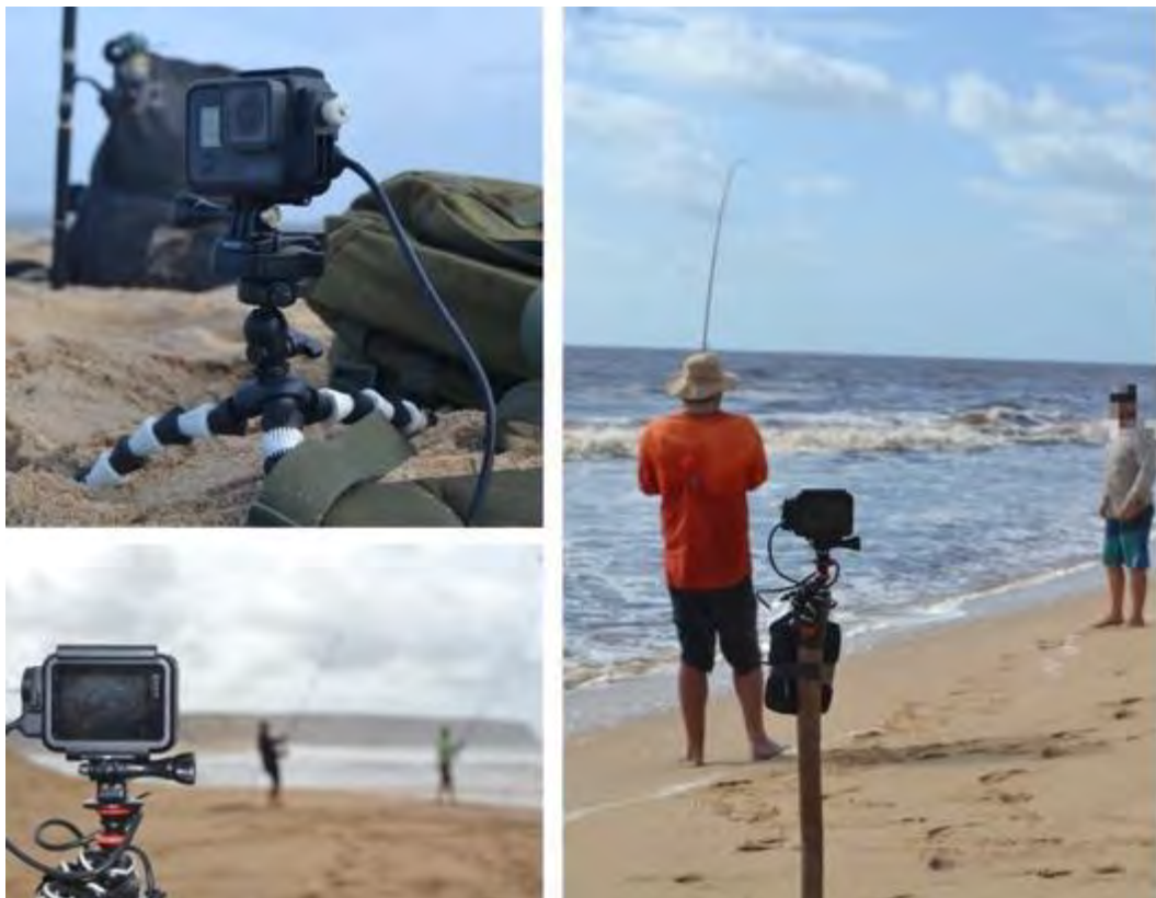
Figure 4.4: Photographs of how the video recording system was deployed to observe catch-and-release events in the recreational shore-based fishery at the mouth of the Longa River, northern Angola.
