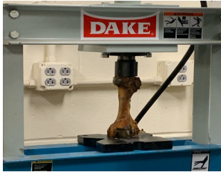
Figure 1. A pig femur bone being crushed in the hydraulic press.
