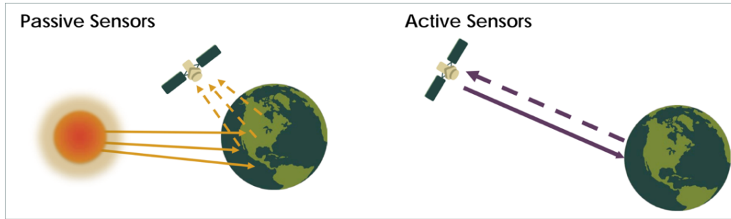
Figure 5. Types of remote sensors. Passive sensors capture reflection of natural light from the object or area of interest. Active sensors provide their own source of light and detect the reflection from the object or area of interest (Credit to NASA Earth Data from the website: https://earthdata.nasa.gov/learn/remote-sensors ).
