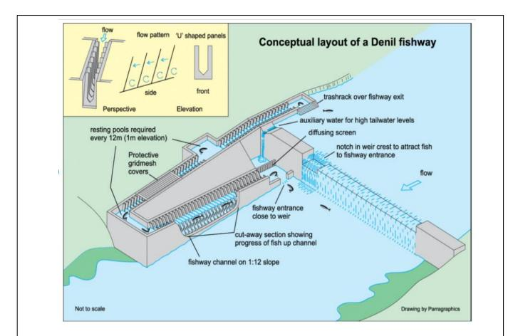
Figure 7: Conceptual layout of a FPD that features a Denil design for upstream passage. Salmon enter from center left entrance at base of dam. Source: https://www.researchgate.net/figure/Conceptual-layout-of-a-Denil-fishway\_fig2\_237346843
