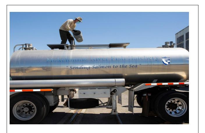
Figure 9: Transport tanker used in CCVR. The tanker is equipped with oxygen and is monitored for appropriate salmon density thresholds. Source: Source: https://www.theguardian.com/us-news/2021/jun/11/california-to-transport-17m-salmon-to-the-sea-by-truck-as-drought-bites
