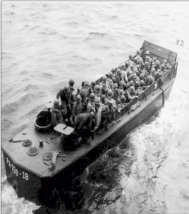
"Higgins Boat": Generally made from plywood, over 20,000 of these amphibious landing crafts were built by Higgins Industries in New Orleans in the early 1940s. Designed with a bow ramp, about 36 troops could disembark quickly to hit the beach when the ramp was lowered. Featured above: USS Darke (APA-159)'s LCVP 18, possibly with army troops as reinforcements at Okinawa, circa 9 to 14 April 1945. US Navy, courtesy Wikimedia.
