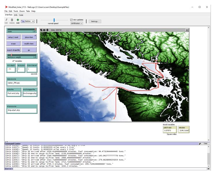
Figure 2.4: Footprints and command centre. Example of footprints created for several ship pathways and multiple anchors. Highlights information gathered in the command centre.
