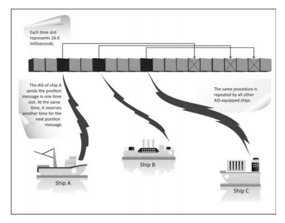
Figure 2.1: SOTDMA protocol for reporting timeslots. Variable timeslots exist depending on the ships sped and where it is going. (Ball, 2013)
