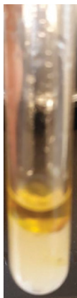
Figure S4. The overall biphasic liquid products collected in the 20-ml sample vial from the experiment to check the mass balance, carbon balance and oxygen balance. Reaction conditions are: pyrolysis temperature was 400 °C, catalytic upgrading temperature was 500 °C, atmospheric pressure, N 2 flow was 1.8 ml min -1 , H-ZSM-5(23) particle size was 300 - 500 μm, glycerol feed was 1 g h -1 , and TOS was 5 h.
