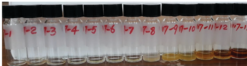
Figure S3. Representative products collected in the 4-ml sample vials at different TOS. Reaction conditions are: pyrolysis temperature was 487 °C, catalytic upgrading temperature was 500 °C, atmospheric pressure, N 2 flow was 1.8 ml min -1 , H-ZSM-5(23) particle size was 500 - 800 μm, and glycerol feed was 1 g h -1 .
