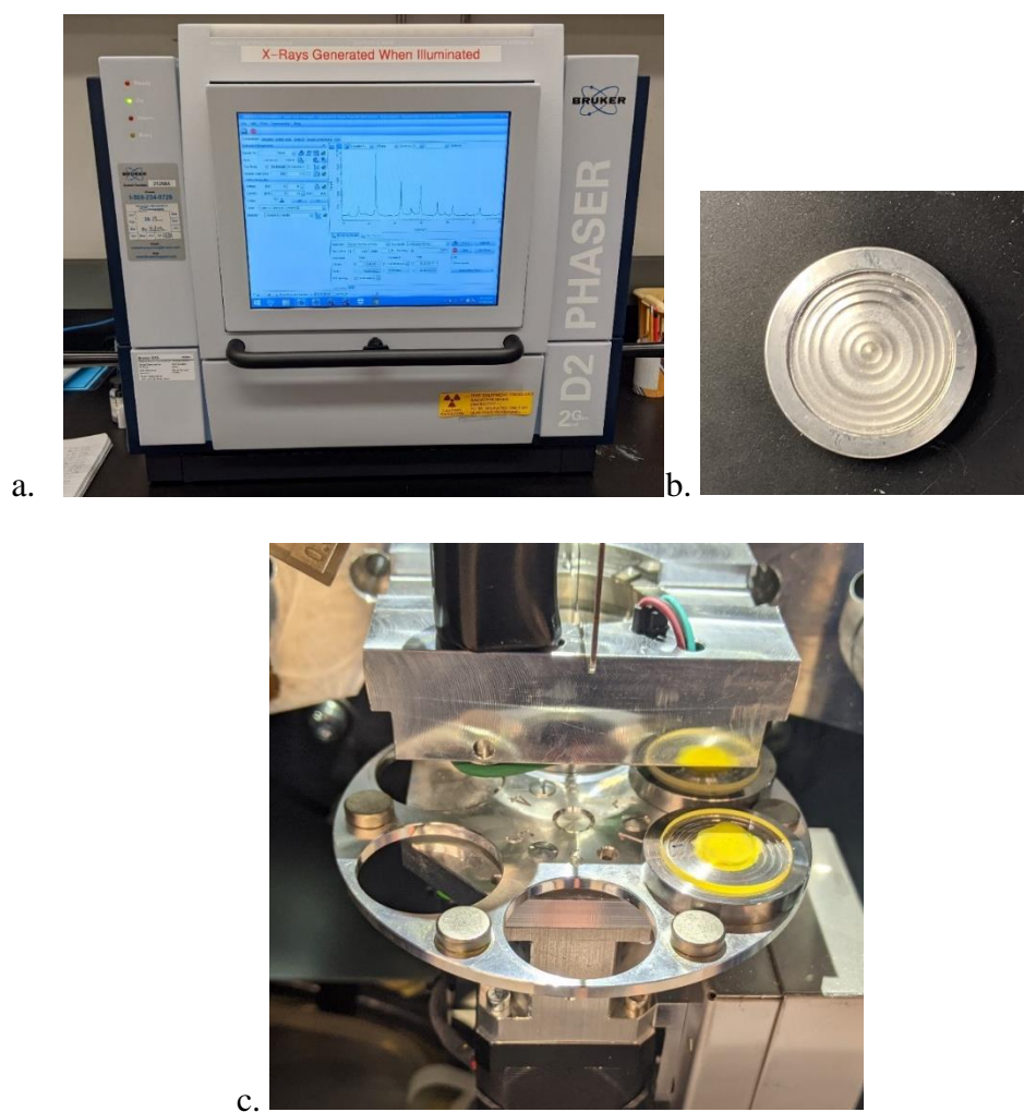
Figure 2-2. a. Bruker D2 Phaser, b. sample holder, and c. inside the Bruker D2 Phaser with two samples.
