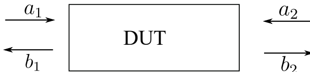
Figure 26: Schematic of a two port device under test (DUT).
