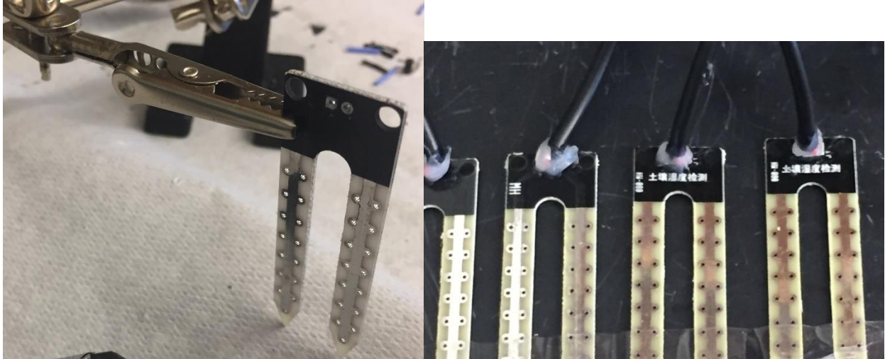
Fig S95. Preparation of soil moisture sensors. Panel A (left) shows removal of pins and solder; panel B (right) shows moisture sensors with new wires attached and waterproof silicone around connections.
