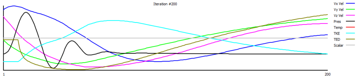
Figure 13. Convergence plot based on CFD simulation of 60 mph wind approaching the eastward oriented system from the west.
