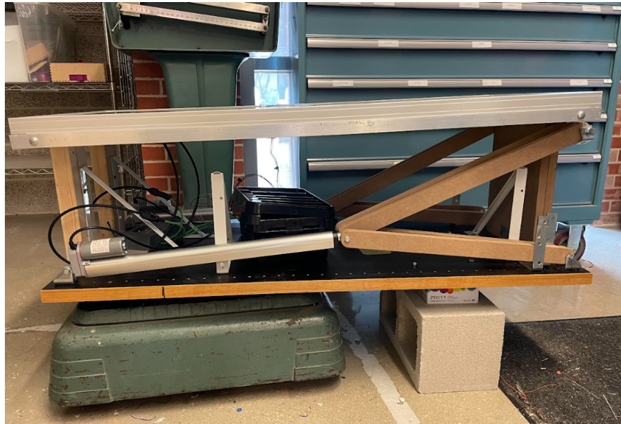
Figure 22. Solar panel system resting flat with one-half on the scale and the other half off.
