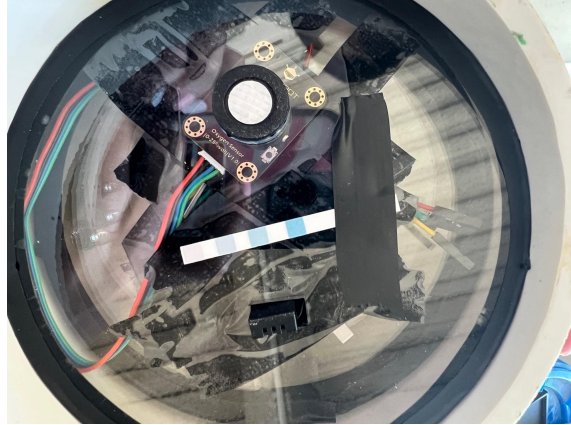
Figure H3. Test strip on the last acrylic membrane near the mesh covering showing about 30% humidity.
