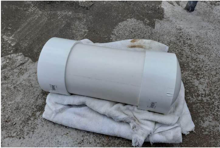
Figure K1. Unblemished sensor capsule prior to impact testing (left) Figure K2. Test setup for the 0.61 m drop (right).
