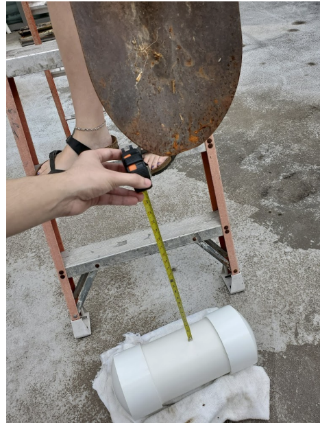
Figure K1. Unblemished sensor capsule prior to impact testing (left) Figure K2. Test setup for the 0.61 m drop (right).
