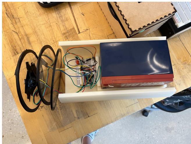
Figure C2. Sub-assembly of the inside of the sensor capsule including the battery, breadboard, and three membranes
