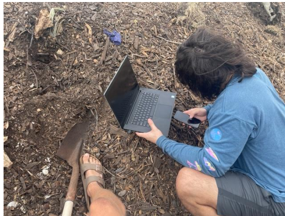
Figure G4. Placing additional pressure on the mass of compost above the sensor capsule while temperature, humidity, and oxygen levels are recorded
