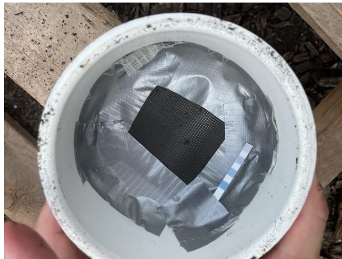
Figure G6. Results of humidity testing - view of test strip placed in the end cap membrane of the device where the sensors rest and are exposed to the ambient environment.
