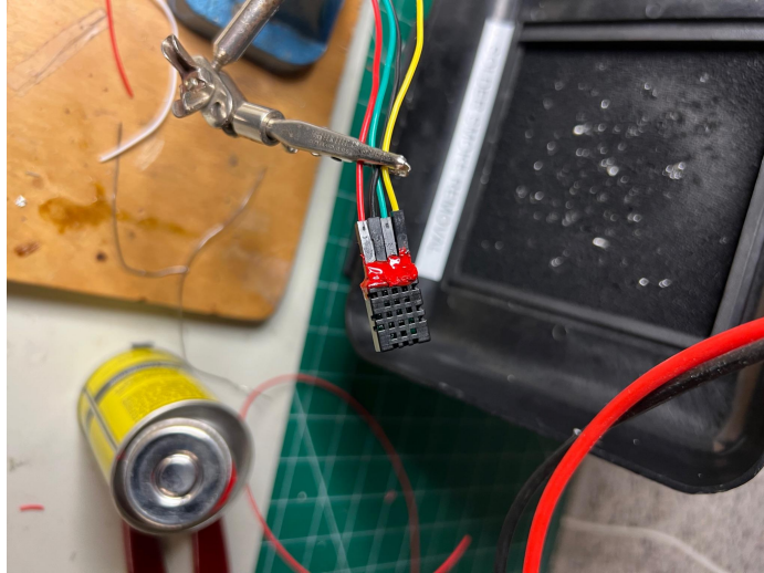
Figure C7. Liquid electrical tape on the temperature & humidity sensor
