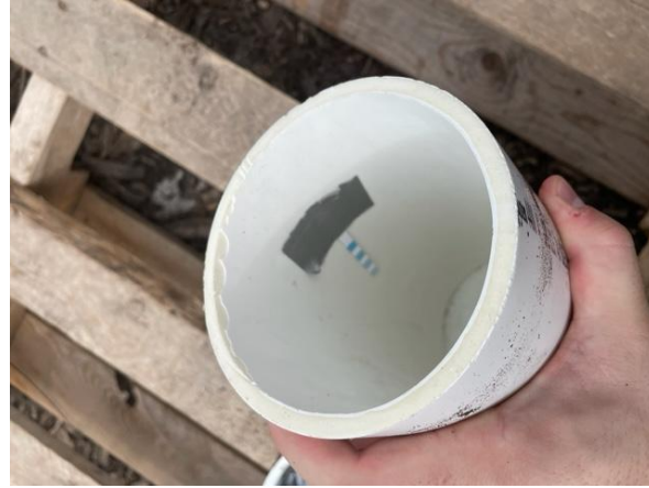
Figure G5. Results of humidity testing at Compost Queens - view of humidity test strip results after capsule was removed from compost. This strip was placed adjacent to where the microcontroller was resting.
