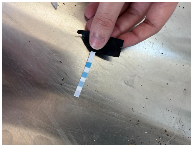
Figure H5. Humidity test strip that was inside with the electronics showing about 15% humidity.
