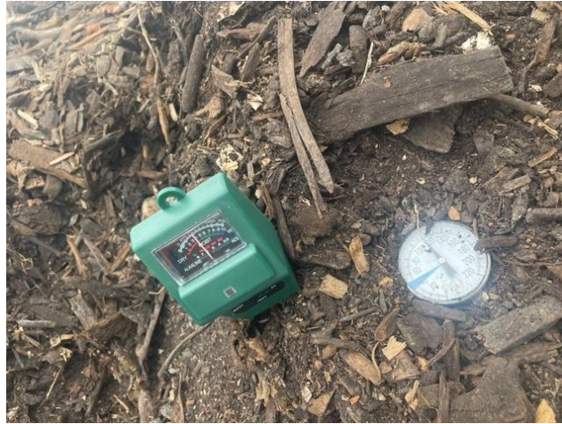
Figure G1. Uncovered handheld probes used for control measurements placed at the top of the compost.
