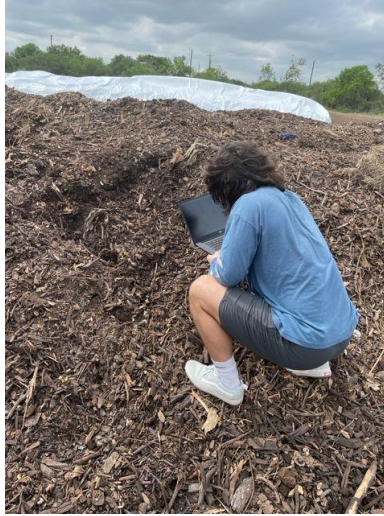
Figure G3. Reading out sensor values from the serial monitor while the peripheral device was covered with mass of compost.
