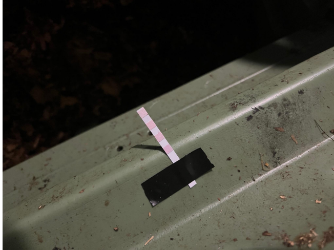
Figure H6. Control humidity test strip that was placed in the compost showing approximately 80% humidity.
