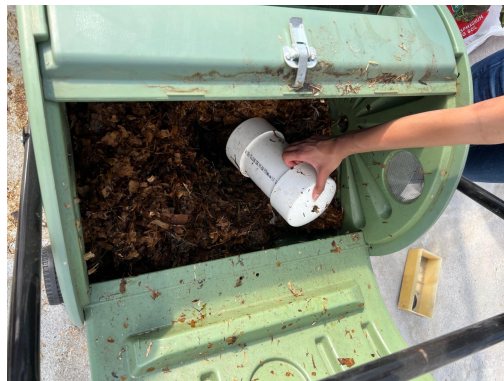
Figure E3. Participant pulling the sensor capsule out of the composting vessel after using a shovel to dig it out.
