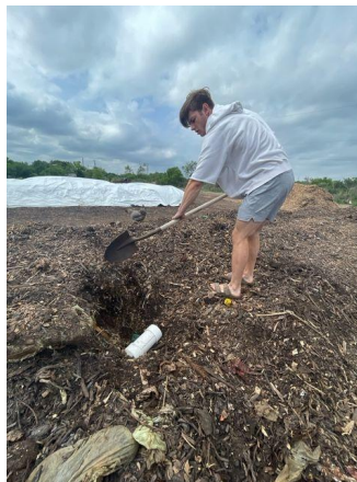
Figure G2. Burying probe under ~3 feet of compost to assess waterproofing and durability of the sensors contained within the capsule as they are exposed to the compost environment.
