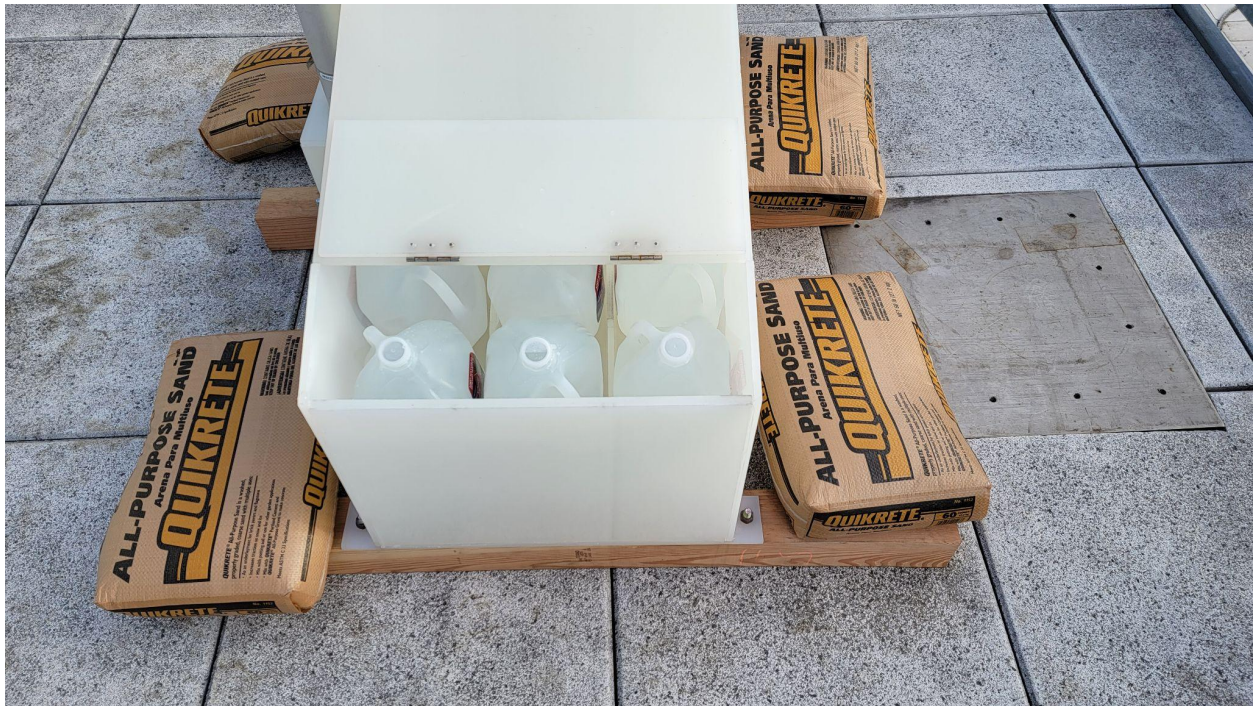
Figure 5.2.1.C. Emergency Water Station 3.0 opening for water jug withdrawals.
