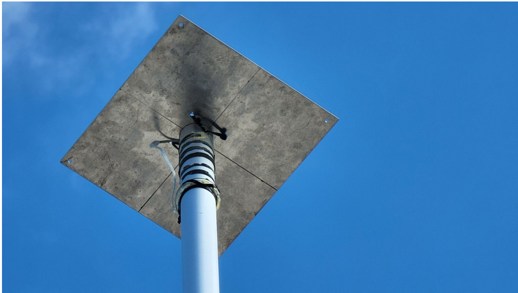
Figure 2.2.G. View of the top of the Emergency Water Station 3.0 pole, where the LED strip has been coiled below the satellite antenna ground plane.
