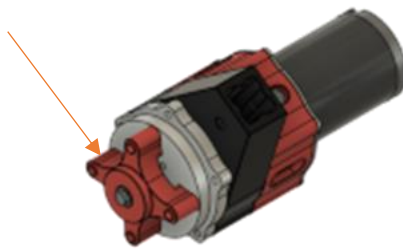
Figure B.1.1 Wheel assembly inherited from summer research team with arrow indicating wheel spacer
