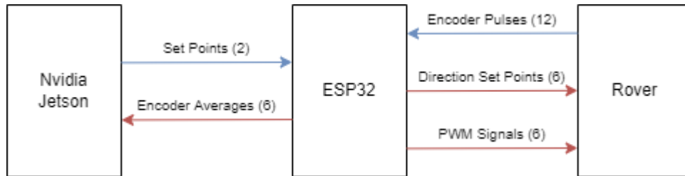
Figure 4. High level I/O flow chart (red – output | blue – input)
