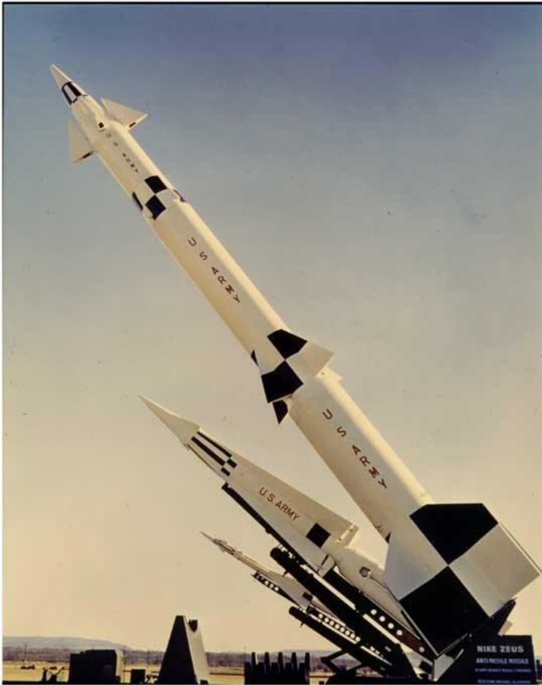
Figure 4: Nike family of missiles. Top to bottom, Zeus, Hercules, Ajax. | Redstone Arsenal Historical Information, U.S. Army, http://www.redstone.army.mil/history/archives/nikefam/nike_family_04.jpg .
