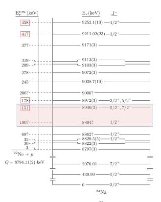
FIG. 1. A diagram of resonant levels in <sup>23</sup>Na in the energy range evaluated in this work. All known spin parities are listed. The energy, spin, and parity of the levels shown as well as the Q value of the <sup>22</sup>Ne( $p,\gamma$ )<sup>23</sup>Na reaction are from Ref. [23]. The center-of-mass interaction energies of the resonances investigated in this work are enclosed in the red boxes. Additionally, the direct-capture reaction rate was measured just below the 417-keV resonance.
