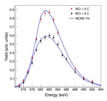
FIG. 5. Typical yield curve of a <sup>22</sup>Ne target used for DC and off-resonance data acquisition before and after 6 C of accumulated beam charge shown as red and black diamonds, respectively.
