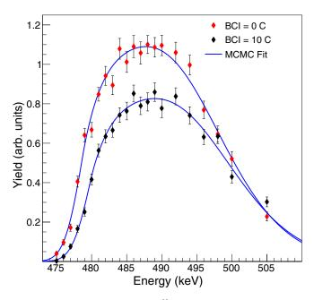
FIG. 4. Typical yield curve of a <sup>22</sup>Ne target used for on-resonance data acquisition before and after 10 C of accumulated beam charge shown as red and black diamonds, respectively.
