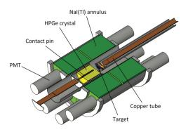
FIG. 2. The LENA  $\gamma\gamma$ -coincidence spectrometer. Original figure from Ref. [32].
