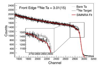
FIG. 3. An example RBS spectrum obtained by measuring  $\alpha$  particles backscattered from a 6.5-keV-thick <sup>22</sup>Ne target is shown in black. A bare tantalum spectrum is shown in gray and a fit to the <sup>22</sup>Ne target data is shown in red. The fit was calculated using the program SIMNRA [41]. A single layer of <sup>22</sup>NeTa in an approximately 1:3 stoichiometry was added onto an infinitely thick Ta sample in SIMNRA was used to obtain the fit to the data.
