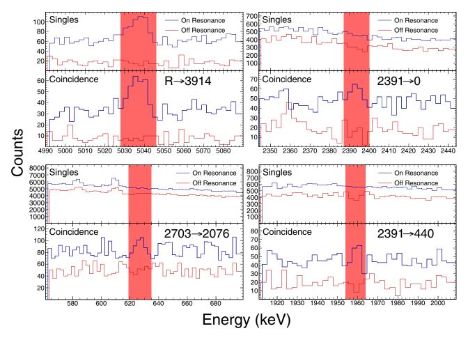
FIG. 15. The singles (top panel) and coincidence (bottom panel) signals from the  $R \to 3914$  transition observed during measurements of the 151-keV resonance in the  $^{22}$ Ne $(p,\gamma)^{23}$ Na reaction. Coincidence off-resonance data are shown on the bottom panel for comparison. The observation of this primary  $\gamma$  ray indicates a significant portion of the observed strength that completely bypasses the 440-keV state.
