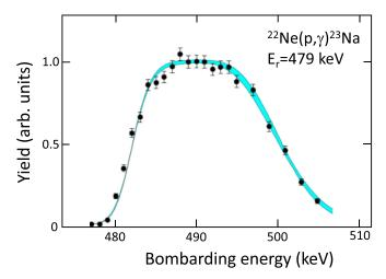
FIG. 1. Yield curve for the  $E_p^{\rm lab}=479~{\rm keV}$  resonance in the  $^{22}{\rm Ne}(p,\gamma)^{23}{\rm Na}$  reaction, after an accumulated  $\alpha$ -particle charge of 3.5 C. The  $\gamma$  ray monitored for the yield had an energy of 6270 keV, corresponding to the 9252  $\rightarrow$  2982-keV primary transition in  $^{23}{\rm Na}$ . The target thickness was about 19 keV for protons at this energy. The cyan-shaded region depicts the uncertainty in the fitted yield curve.
