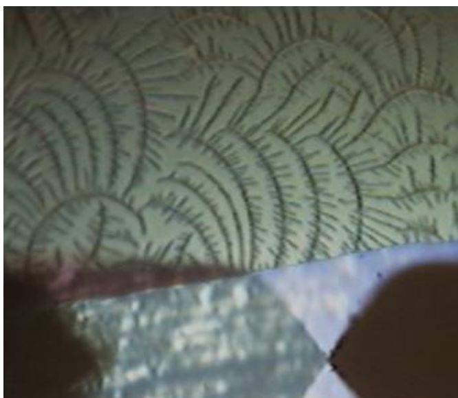
Figure S3.19. Crystallites observed on the surface of P3HT:3TZA:PC 61 BM 1:0.8:1 films cast from oDCB.
