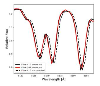
**Figure 7.** Illustration of the improvement in blue arm wavelength calibration around the Mgb 5177 Å lines. The black solid and dashed lines show a corrected and uncorrected twilight sky spectrum from fibre 410. The solid red line shows a wavelength corrected spectrum from fibre 397. After wavelength correction the agreement between different fibres is significantly improved.
