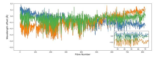
Figure 6. The measured wavelength offset with respect to a high-resolution solar spectrum in Å as a function of fibre number for three twilight sky observations (indicated by the three different colours). The inset shows a zoom in over a small range of fibres to better illustrate the fibre-to-fibre variation.
