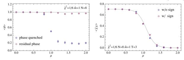
FIG. 4. Left: Phase average in for real phase quenched simulations and the average of the residual phase for single thimble simulations. Right: the chiral condensate with and without the residual phase folded in. The solid line represents the exact result that includes contribution from other thimbles.
