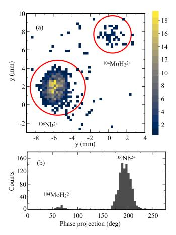
FIG. 1. Example CPT spectra acquired using the PI-ICR technique with  $t_{\rm acc}=190\,$  ms. (a) Ions acquire a mass-dependent phase, forming characteristic "spots," during the collection time in the trap. The  $^{106}{\rm Nb}^{2+}$  and molecular  $^{104}{\rm MoH_4}^{2+}$  are identified. (b) Corresponding phase projection of  $^{106}{\rm Nb}^{2+}$  and the  $^{104}{\rm MoH_4}^{2+}$  contaminant.
