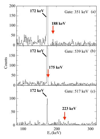
FIG. 9. Background-subtracted projection of the  $\beta$ -gated,  $\gamma$ - $\gamma$ -coincidence matrix, gated on the (a) 351-keV (4<sup>+</sup>  $\rightarrow$  2<sup>+</sup>), (b) 539-keV (2<sup>+</sup>  $\rightarrow$  2<sup>+</sup>), and (c) 517-keV (J<sup> $\pi$ </sup>  $\rightarrow$  5<sup>+</sup><sub>(1)</sub>) transitions in <sup>106</sup>Mo, from 100 to 300 keV. Expected locations of the unobserved  $\gamma$  rays from Ref. [5] are indicated by the red arrows and discussed in the text.
