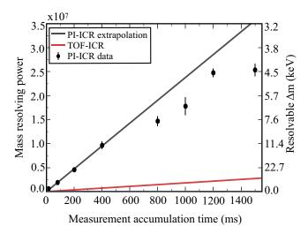
FIG. 2. Mass resolving power and resolvable mass differences with the PI-ICR technique (black line) as a function of accumulation time  $t_{\rm acc}$ . For comparison, the achievable resolving power with the Time-of-Flight Ion-Cyclotron-Resonance (TOF-ICR) technique (red line) is also shown.
