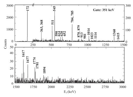
FIG. 6. Background-subtracted,  $\beta$ -gated,  $\gamma$ - $\gamma$ -coincidence matrix, gated on the well-known 351-keV ( $4_1^+ \rightarrow 2_1^+$ ) transition in  $^{106}$ Mo, from (top) 0 to 1500 keV, and (bottom) 1500 to 3000 keV. The  $\gamma$  rays from transitions in  $^{106}$ Mo are labeled with their energies. Note the change of  $\gamma$ -axis scale at 250 keV in the top panel.
