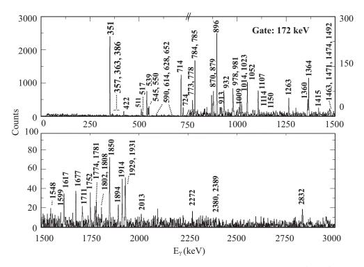
FIG. 5. Background-subtracted,  $\beta$ -gated,  $\gamma$ - $\gamma$ -coincidence matrix, gated on the well-known 172-keV ( $2_1^+ \to 0_1^+$ ) transition in  $^{106}$ Mo, from (top) 0 to 1500 keV, and (bottom) 1500 to 3000 keV. The  $\gamma$  rays from transitions in  $^{106}$ Mo are labeled with their energies. Note the change of y-axis scale at 750 keV in the top panel.
