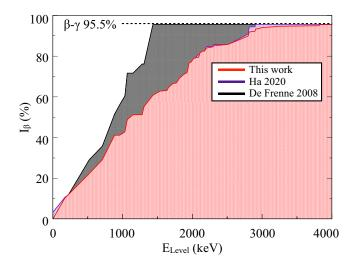
FIG. 4. Accumulation of the apparent  $\beta$ -feeding strength of  $^{106}$ Nb as a function of excitation energy of the decay progeny,  $^{106}$ Mo, from this work (red), Ha *et al.* [5] (purple) and derived from  $\gamma$ -ray intensities given in the most-recent data evaluation [16] (black). A  $\beta$ -delayed neutron branch of 4.5(3)% for  $^{106}$ Nb is assumed [16].
