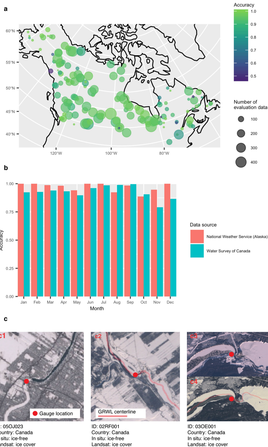
Extended Data Fig. 9 | Evaluating Landsat-derived river ice conditions against in situ river ice records. a , The accuracy of Landsat-derived river ice extents when evaluated against in situ reports of river ice condition. b , Monthly evaluation of Landsat-derived river ice estimates. c , Examples of differences in
