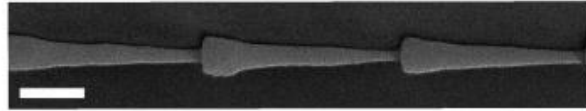
Figure 3.5: Sawtooth sections in series. SEM image of a NW with three geometric diodes encoded in series; scale bar, 200 nm.
