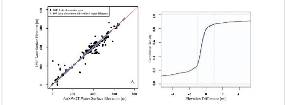
Figure 5. Black dots in (A) and line in (B) show AirSWOT vs. LVIS WSE after adding the MERIT reference elevation filter, using all 1043 available AirSWOT-LVIS lake observation pairs. Blue dots (A) and line in (B) show AirSWOT WSE vs. LVIS WSE after reference elevation filtering and limiting the absolute difference between AirSWOT and LVIS to 1 meter using 805 available AirSWOT-LVIS lake pairs.
