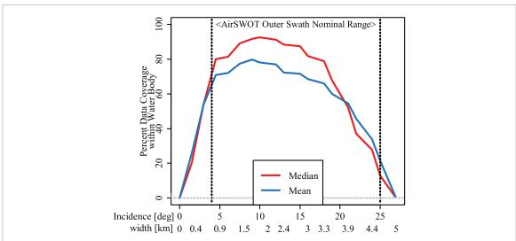
**Figure 2.** Approximately 70% of the AirSWOT radar data are recovered within the nominal swath range, with rapid data loss <4° and >17°. WSE data is present mostly at >4 degrees of incidence.
