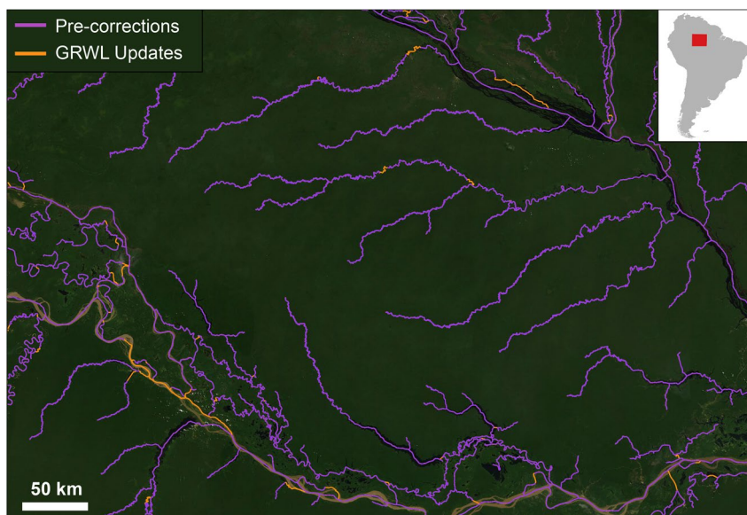
Figure 2. Example of GRWL centerline corrections along the Amazon River. Purple lines represent the GRWL centerlines before corrections, and orange lines represent the centerline updates. Upper right inset shows the selected location in South America.
