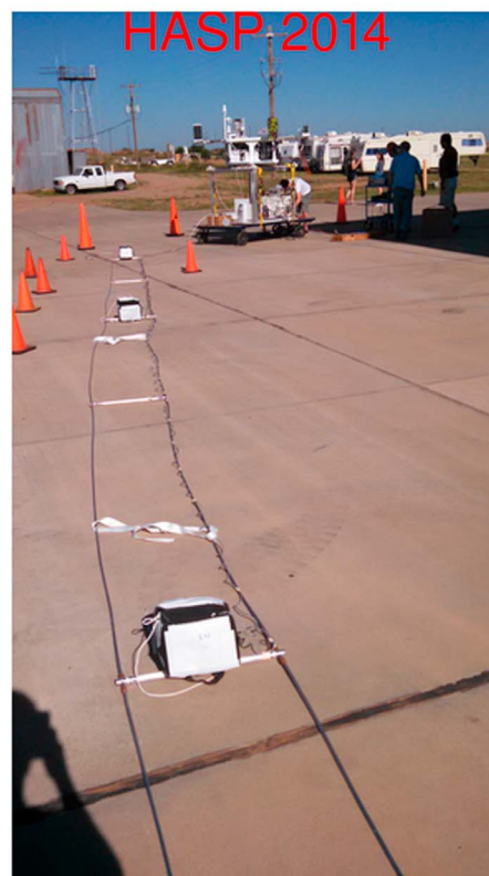
Figure 1. Infrasound microphone layout on the (top) HASP 2014 and 2015, (bottom left) the HASP 2014 flight ladder microphone array during a ground test, and (bottom right) the HASP 2015 balloon at neutral buoyancy in the stratosphere. Note that station GOND on the HASP 2015 was located on the instrumented gondola below the flight ladder.
