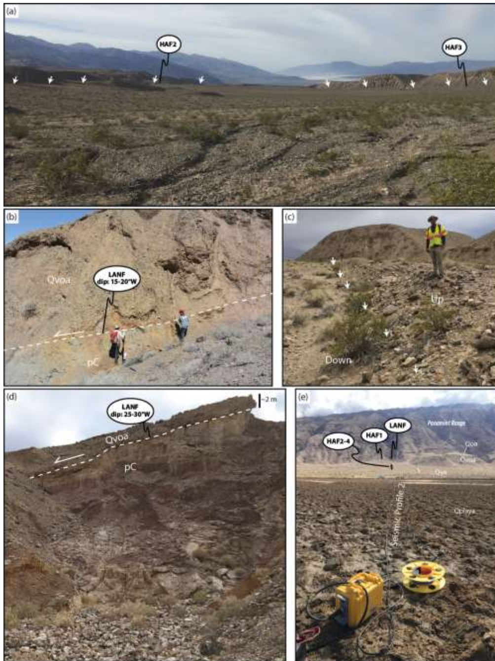
Figure 6. Field photographs. (a) Overview of Wildrose graben, looking south. High-angle faults, HAF2 (synthetic) and HAF3 (antithetic), define the margins of the graben and are indicated by white arrows. (b) Low-angle normal fault (LANF) characterized by fault gouge in exposure near Wildrose graben, separating Plio-Pleistocene alluvial fan material (Qvoa) from Proterozoic metasedimentary deposits (pC). (c) Youthful scarp in the axis of Wildrose graben indicated by white arrows. (d) LANF in exposure at east termination of Profile 2, dipping 25-30° to the west and separating Plio-Pleistocene alluvial fan material (Qvoa) from Proterozoic mylonitic leucogranite (pC). (e) Overview of Profile 2, looking east across the playa (Qplaya) and toward the Panamint Range. Location and view directions of photographs (a-c) indicated in Figure 3a and (d-e) in Figure 5a. Photographs taken April–May 2018 by R. Gold.
