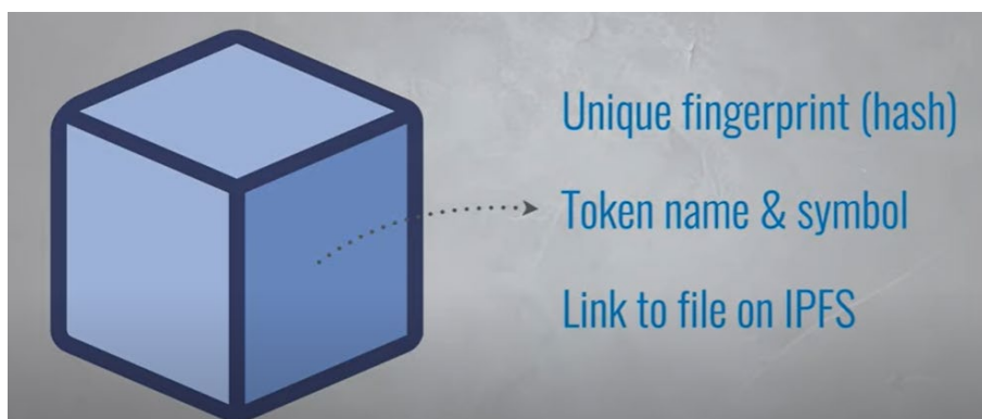
Figure 2: A representation of an NFT block, and comprises it. The unique fingerprint hash is similar to a hash within any other type of block, as is the parent hash of the previous block. The token name, symbol, and (optionally) link to the data the NFT represents on IPFS (Interplanetary File System) comprise the data component of the block. (Simply Explained, 2021).
