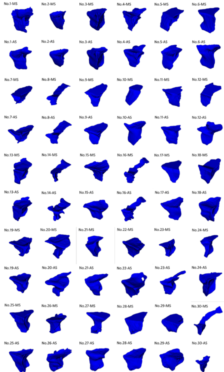
Figure 14. Defect renderings using 3D imaging software. Both manual segmentation (MS) and automatic segmentation (AS) results are shown.
