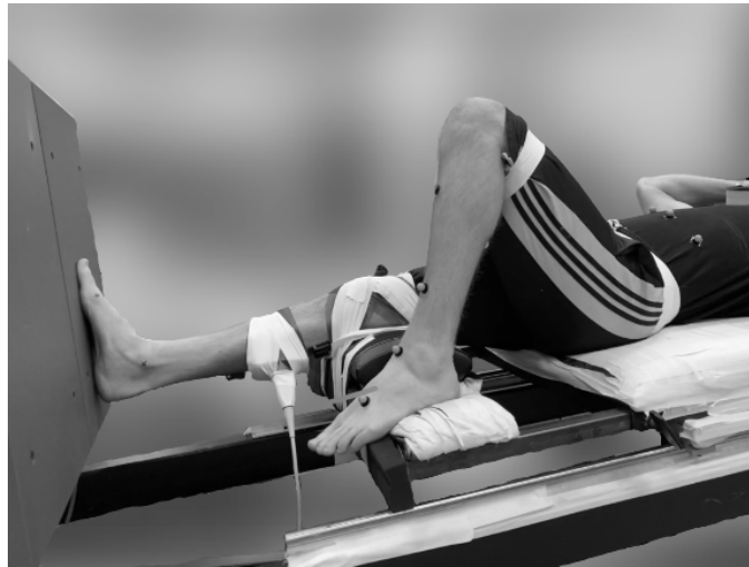
Figure 1. Image of a subject on the carriage. Their right knee is immobilized with their right calf fitted with an ultrasound probe and their lower body has 16 retro-reflective markers placed in anatomical positions
