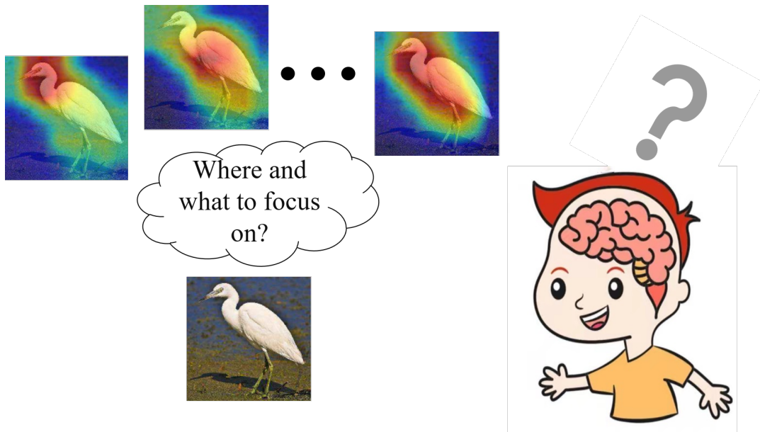
Figure 1.2: The visual attention mechanism mimics the human’s perception process. The attention mechanism can localise the informative regions within the image. It thereby helps the deep network to encode a discriminative feature embedding for the input image. In the heat map, the response increases from blue to red. Best viewed in colour.
