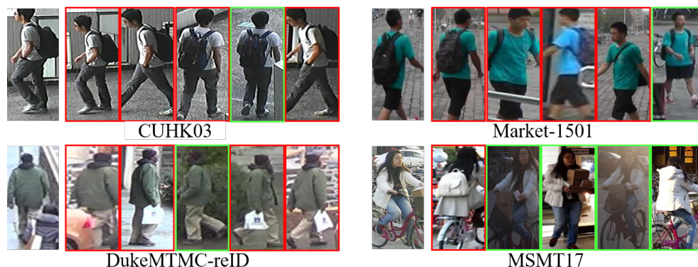
Figure 3.10: Some failure cases on person re-ID datasets. In each ranking list, to the left is the query person and to the right is the corresponding ranked list in the gallery set. The correct and false matches are enclosed in green and red boxes. Best viewed in colour.
