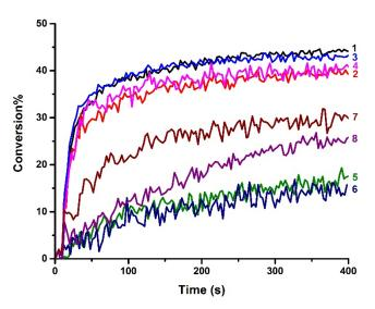
**Figure 3.** Photopolymerization profiles of EPOX (epoxy function conversion vs. irradiation time) upon LED@365 nm irradiation under air in the presence of (1) BPC1/Iod  $(0.5\%/1\% \ w/w)$ ; (2) BPC2/Iod  $(0.5\%/1\% \ w/w)$ ; (3) BPC3/Iod  $(0.5\%/1\% \ w/w)$ ; (4) BPC4/Iod  $(0.5\%/1\% \ w/w)$ ; (5) C5/Iod  $(1\%/1\% \ w/w)$ ; (6) C6/Iod  $(0.5\%/1\% \ w/w)$ ; (7) C7/Iod  $(0.5\%/1\% \ w/w)$ ; (8) C8/Iod  $(0.5\%/1\% \ w/w)$ . The irradiation starts from t = 10 s.
