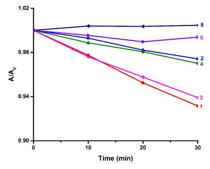
**Figure 6.** Photolysis kinetics of PI/TEOA systems upon LED@375 nm irradiation in acetonitrile (1) BPC1/TEOA, (2) BPC2/TEOA, (3) BPC3/TEOA, (4) BPC4/TEOA, (5) C5/TEOA, (6) C7/TEOA. ( $A_0$  absorbance of maximum wavelength at t min.).
