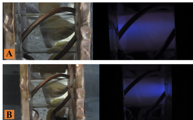
FIG. 8. The images of the produced blue core in m = -1 (a) and m = +1 (b) helicon modes recorded using a camera with polarizing filters at 900 W RF power, 300 mT magnetic field intensity, and 3 SCCM argon flow rate.
