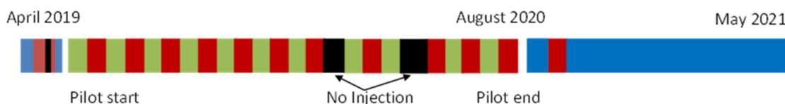
**Figure 6.** Injection overview of the radial model for East Seminole Field. Water injections (blue), CO<sub>2</sub> injections (red), surfactant injections (green), no injection periods (black).
