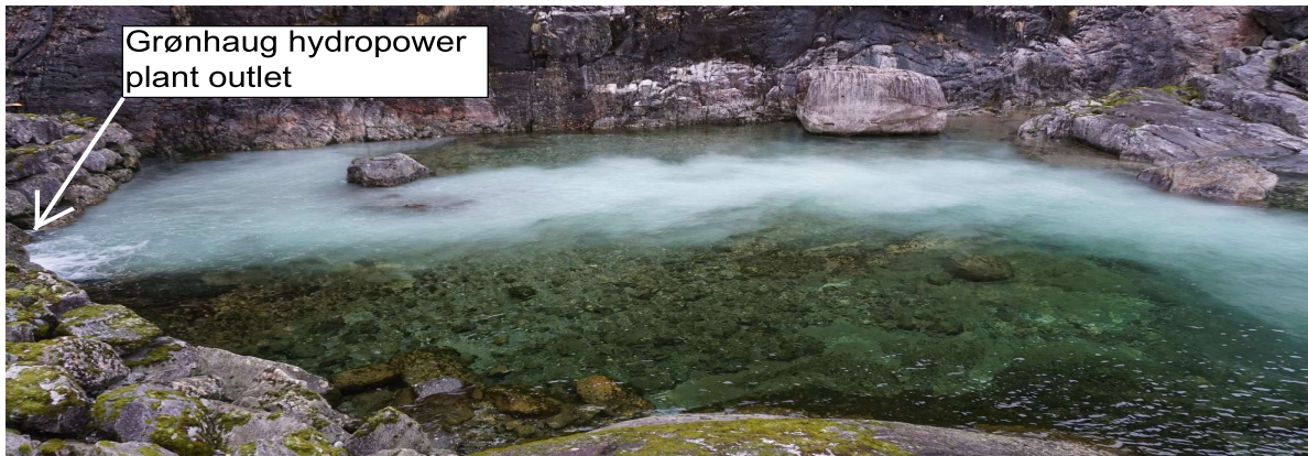
(a) Visible sign of TDG supersaturation during field tests November 2021
