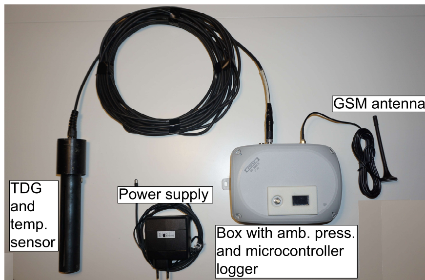
Figure 3.3: TDG sensor with logger junction box, GSM antenna and power supply
