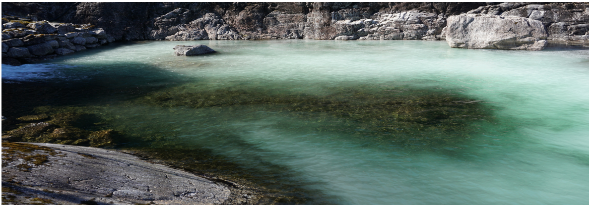
(b) Visible sign of TDG supersaturation during field tests April 2022
