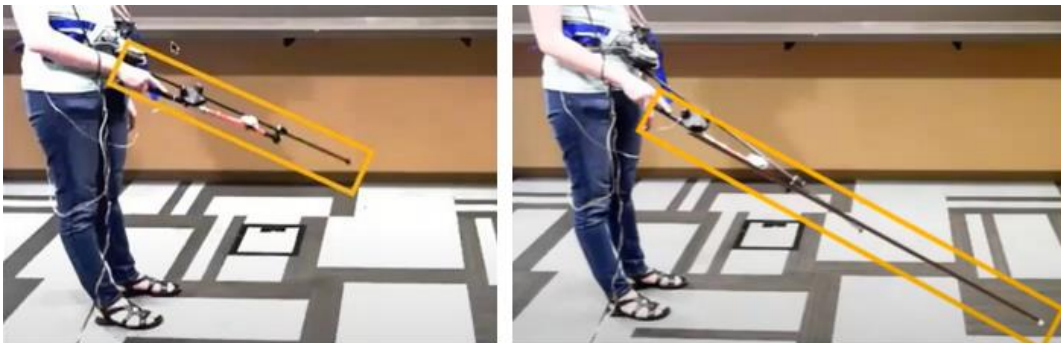
Figure 5.3a – Cane controller seen in real life (short) Figure 5.3b – Cane controller seen in VR (actual size of a cane) (XR Access, 2021)
