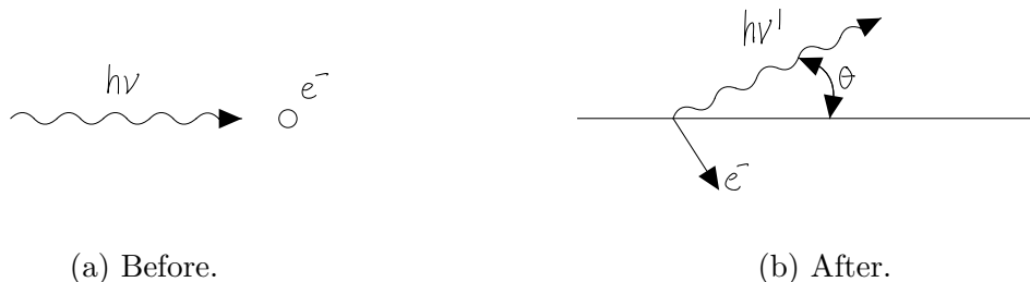
Figure 3.13: Diagram of compton scattering interaction between gamma-ray and electron. Adopted from [14].
