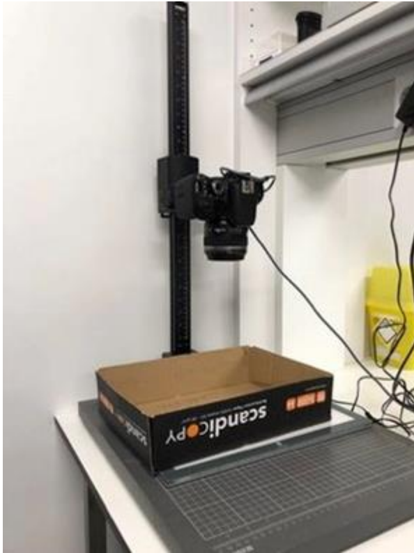
Figure 2. Camera set up for photographs of salmon lice picked off fish temporarily. Camera mounted on a stand at 45.5cm. A cut cardboard box with a hole for placing the Petri dish with salmon lice is placed under the camera and back lit from an external source.
