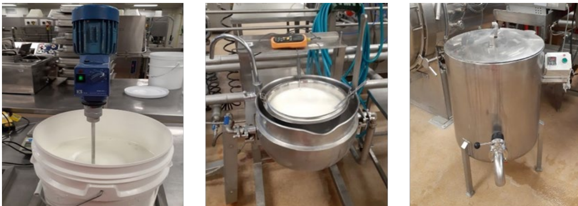
Figure 5.1 Fermented milk for the consumer study prepared at the Massey University Food Pilot Plant. Milk was reconstituted by mixing skim milk powder and water using an overhead stirrer (a). The milk was heat-treated using a steam kettle to rapidly heat the milk to 85\text{ }^{\circ}\text{C} (b). The milk was then held in a water-jacketed kettle, set to 85\text{ }^{\circ}\text{C} for 30 mins. Fermentation took place in the water-jacketed kettle (c).
