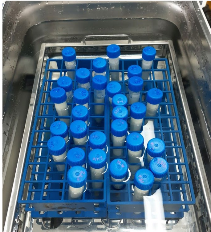
Figure 4.2 Placement of tubes/fermented milk in the water bath. The position of each tube in the water bath was randomised according to the experimental design prepared in CycDesignN. Each tube corresponds to a different starter/probiotic/fermentation time point.
