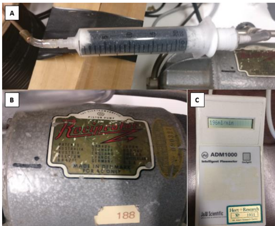
Figure 3.3: (A) activated charcoal filter, (B) Reciprotor electromagnetic piston pump, and (C) airflow meter
