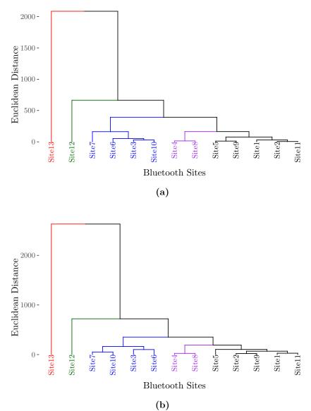
Figure 2.7: The dendrogram of Bluetooth site clustering based on two variables: i) the total number of Bluetooth detections; and ii) the total number of unique Bluetooth MAC addresses using the average linkage and Euclidean distance between (a) 3:00-4:00 p.m. and (b) 4:00-5:00 p.m., Monday 11th February 2019. The five clusters are represented by different colors.
