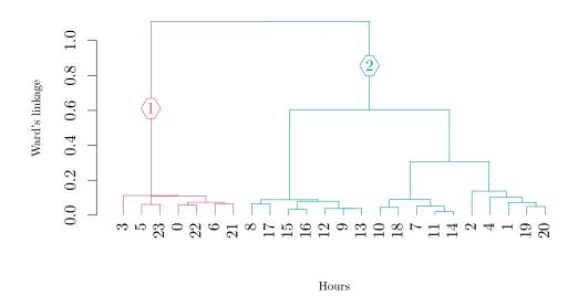
Figure A.17: The dendrogram of time interval clustering based gap distribution using Ward linkage and KS distance at Site 12, Wednesday 13th February 2019.
