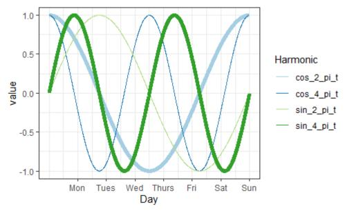
Figure 4.3: The four Fourier harmonic basis functions by considering m = 2. The highlighted blue and green harmonic functions are corresponding to the cosine and the sine term for k = 1 and k = 2, respectively.
