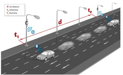
Figure 1.6: The operational concept of collecting traffic data using Bluetooth detectors (Source:www.libelium.com).
