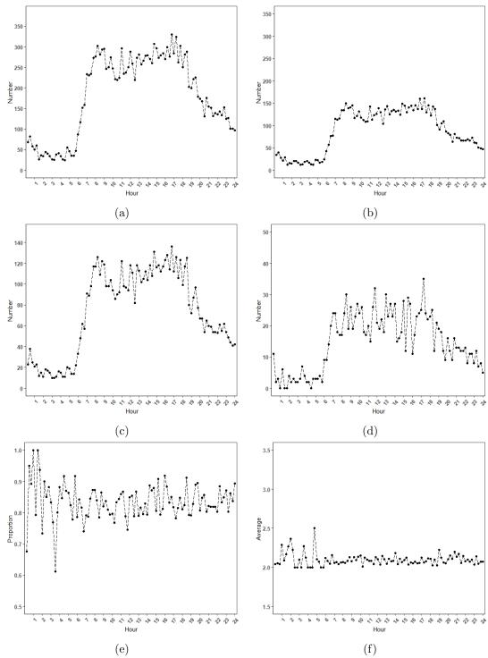
**Figure A.4:** Hourly patterns for the first four considered variables: (a) the number of all recorded of MAC addresses detected, (b) the number of all unique MAC addresses detected, (c) the number of MAC addresses with multiple detections, (d) the number of MAC addresses with only one detection, (e) the proportion of MAC addresses with multiple detections, and (f) the average number of detections for the MAC addresses with multiple detections at Site 12, Friday 15 February, 2019.
