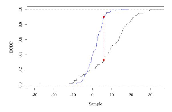
Figure 2.10: An example of the two-sample KS statistic. The dashed red line is the two-sample KS statistic (i.e. maximum distance D), and the blue and black lines represent the empirical distribution function for two samples.
