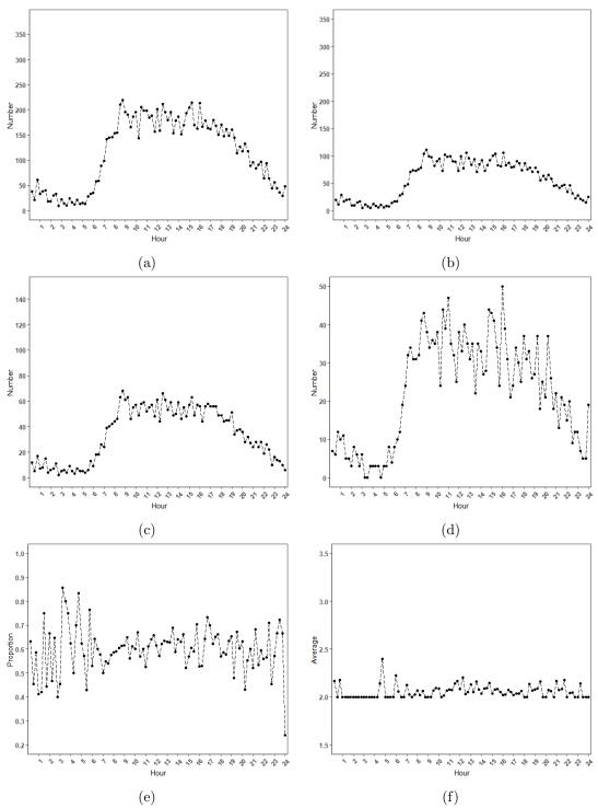
**Figure A.9:** Hourly patterns for the first four considered variables: (a) the number of all recorded of MAC addresses detected, (b) the number of all unique MAC addresses detected, (c) the number of MAC addresses with multiple detections, (d) the number of MAC addresses with only one detection, (e) the proportion of MAC addresses with multiple detections, and (f) the average number of detections for the MAC addresses with multiple detections at Site 6, Monday 11 February, 2019.
