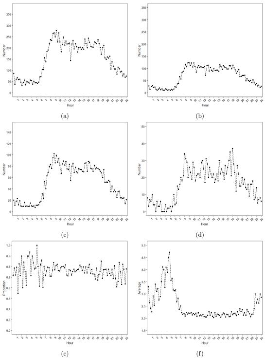
**Figure A.10:** Hourly patterns for the first four considered variables: (a) the number of all recorded of MAC addresses detected, (b) the number of all unique MAC addresses detected, (c) the number of MAC addresses with multiple detections, (d) the number of MAC addresses with only one detection, (e) the proportion of MAC addresses with multiple detections, and (f) the average number of detections for the MAC addresses with multiple detections at Site 7, Monday 11 February, 2019.
