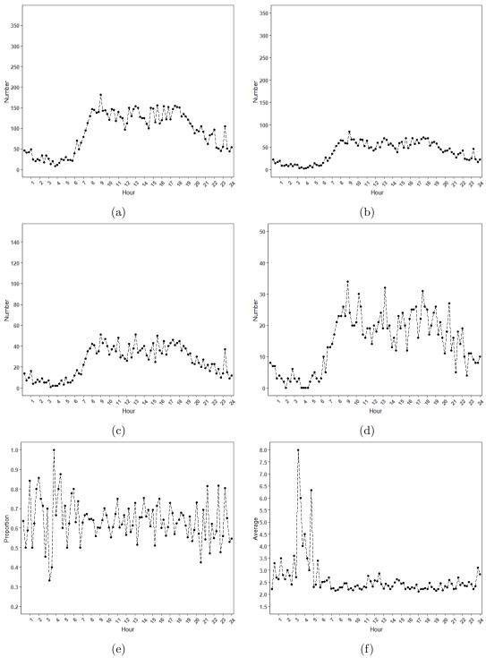
**Figure A.6:** Hourly patterns for the first four considered variables: (a) the number of all recorded of MAC addresses detected, (b) the number of all unique MAC addresses detected, (c) the number of MAC addresses with multiple detections, (d) the number of MAC addresses with only one detection, (e) the proportion of MAC addresses with multiple detections, and (f) the average number of detections for the MAC addresses with multiple detections at Site 1, Monday 11 February, 2019.
