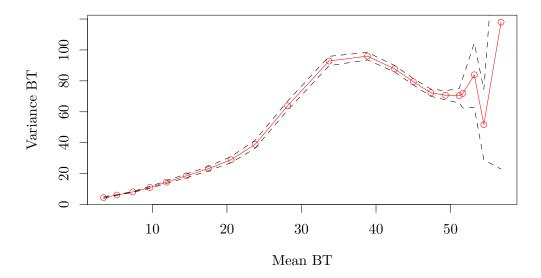
Figure 3.4: The variance versus the mean of Bluetooth detections across the rolling windows of ATC counts for location 2. The estimates from each window are shown as circles, with bootstrap 95% confidence limits as dashed lines.
