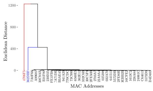
Figure 2.9: The dendrogram of MAC addresses clustering at Site 13 based on two variables: i) the number of all detections per MAC addresses; and ii) the mean of the gap times for each MAC address. It creates using the average linkage and Euclidean distance and displays for time period 3:00-4:00 a.m., Monday 11th February 2019.
