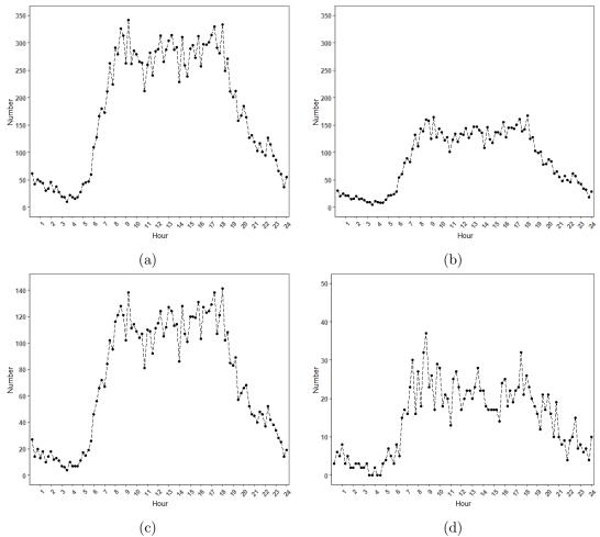
Figure 2.2: Hourly patterns for the first four considered variables: (a) the number of all recorded of MAC addresses detected, (b) the number of all unique MAC addresses detected, (c) the number of MAC addresses with multiple detections, and (d) the number of MAC addresses with only one detection on Site 12, Monday 11th February, 2019.
