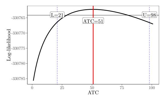
Figure 4.16: The calibration result using the profile log-likelihood where the number of Bluetooth counts is assumed to be 19 in the five minute time interval between 17:05-17:10 on Monday. The vertical red and the dashed blue lines mark the optimum value and the confidence calibration intervals, respectively.
