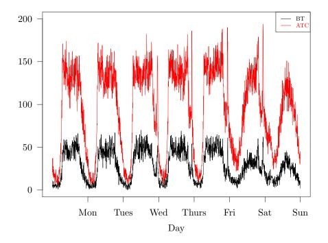
Figure 4.2: Bluetooth and ATC record data in five minutes time interval for one week, 22-28 January, 2018.
