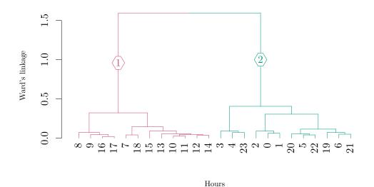
Figure 2.13: The dendrogram of time interval clustering based gap distribution using Ward's linkage and KS distance at Site 12, Monday 11th February 2019.
