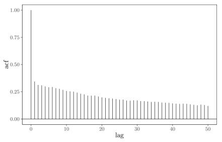
Figure 3.11: The autocorrelation of the residuals from the weighted segmented regression model with two knots for location 2.
