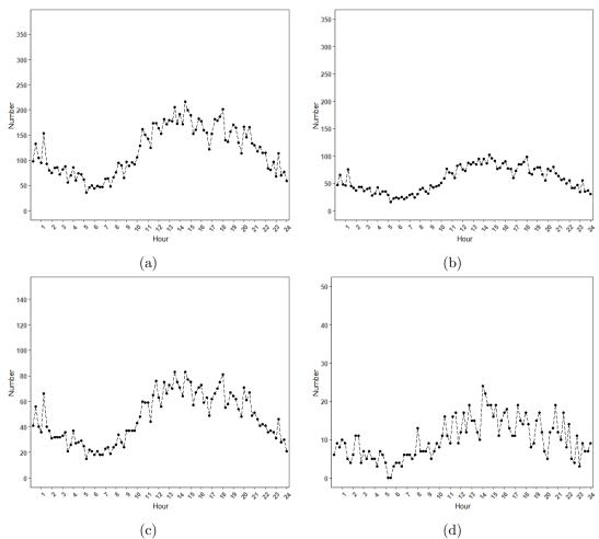
Figure 2.4: Hourly patterns for the first four considered variables: (a) the number of all recorded of MAC addresses detected, (b) the number of all unique MAC addresses detected, (c) the number of MAC addresses with multiple detections, and (d) the number of MAC addresses with only one detection at Site 12, Sunday 17 February, 2019.
