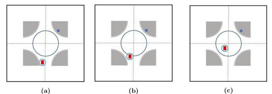
**Figure 1.5:** (a) The car is outside of the Bluetooth pick-up area; (b) the car is partially in the pick-up area; (c) the car is now fully in the pick-up area.
