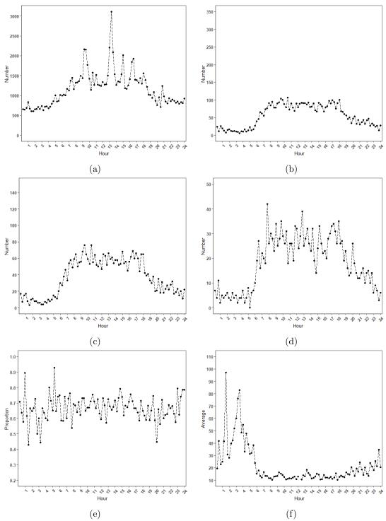
**Figure A.14:** Hourly patterns for the first four considered variables: (a) the number of all recorded of MAC addresses detected, (b) the number of all unique MAC addresses detected, (c) the number of MAC addresses with multiple detections, (d) the number of MAC addresses with only one detection, (e) the proportion of MAC addresses with multiple detections, and (f) the average number of detections for the MAC addresses with multiple detections at Site 13, Monday 11 February, 2019.
