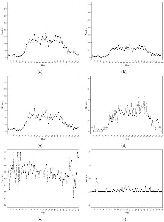
**Figure A.13:** Hourly patterns for the first four considered variables: (a) the number of all recorded of MAC addresses detected, (b) the number of all unique MAC addresses detected, (c) the number of MAC addresses with multiple detections, (d) the number of MAC addresses with only one detection, (e) the proportion of MAC addresses with multiple detections, and (f) the average number of detections for the MAC addresses with multiple detections at Site 11, Monday 11 February, 2019.
