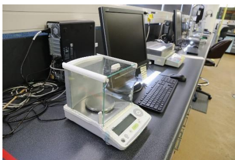
Figure 3.2. Weight loss measurement (A digital balance (S-4002, Denver instruments, Colorado, USA, with a precision of 0.001g).
