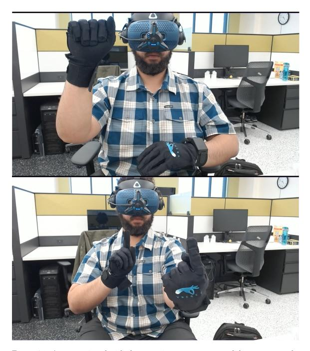
Figure 4.1: A user equipped with the two primary components of the apparatus: the Vive Cosmos VR Headset, and the VRFree Gloves.
