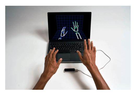
Figure 2.13: A user's hands being tracked by the LEAP motion device and the resulting skeletal figures provided by the accompanying SDK [37].
