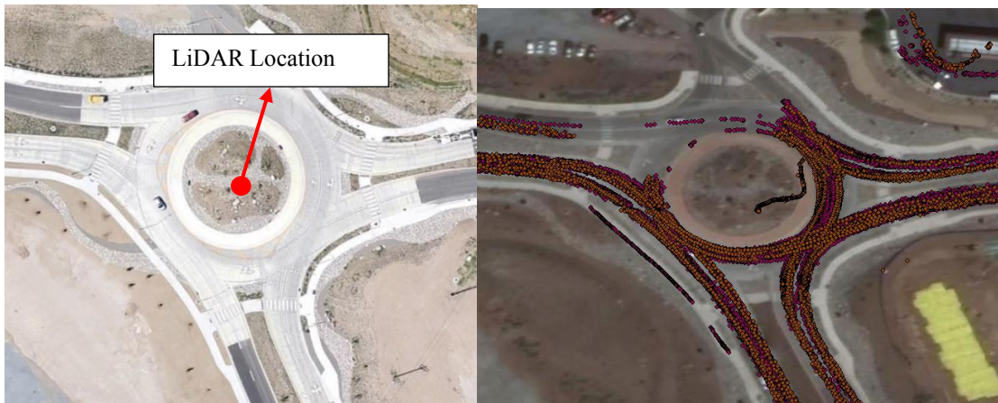
Figure 7 (left) Study Roundabout and LiDAR Locations and (right) Georeferenced LiDAR trajectory Results
