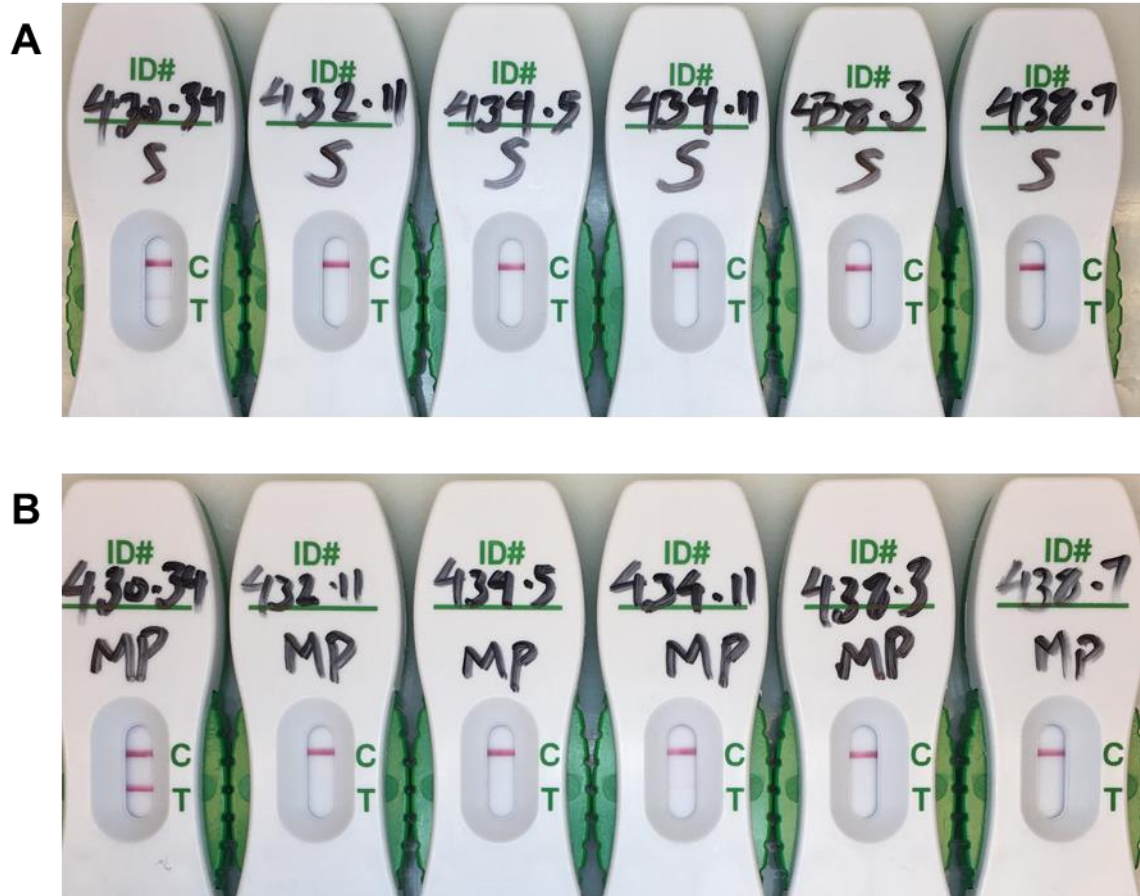
Figure 4. Images of AMD Plus LFI results from testing the human melioidosis samples obtained from Menzies School of Health Research. (A) Results from testing the samples using the standard testing protocol where sample ID 430-34 and 434-11 were positive. (B) Results from testing the samples using the magnetic immunoprecipitation protocol where sample ID 430-34, 432-11, 434-11, 438-3, and 438-7 were positive.
