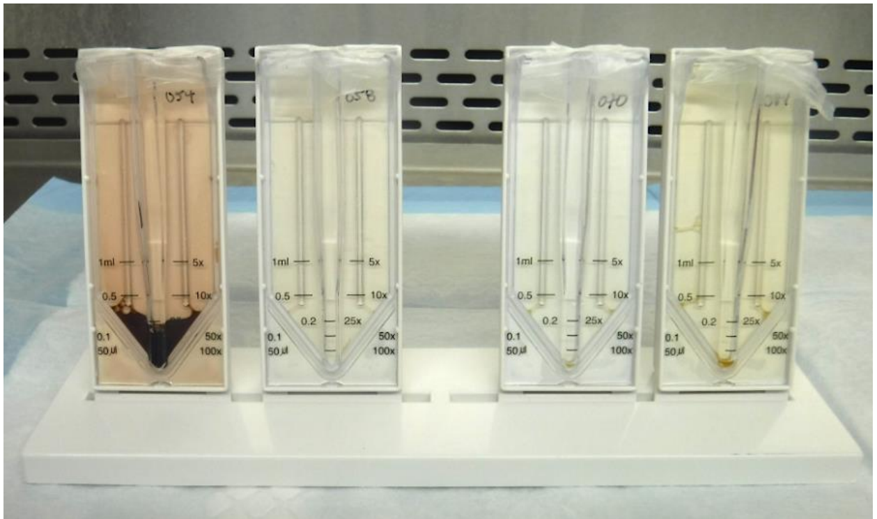
Supplemental Figure 1. Image of Vivapore BJP-5/30 concentrators used for concentrating urine samples from melioidosis patients. Sample MRDT-054 did not fully concentrate and appears to contain a substantial amount of red blood cells.
