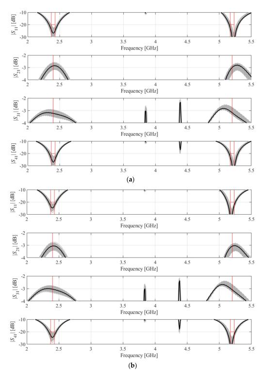
**Figure 7.** EM-driven Monte Carlo simulation of Circuit III (Figure 3c) at (**a**) the nominal design, and (**b**) the final design obtained using the proposed algorithm. MC carried out using 500 random samples. EM simulation data shown as gray curves. Black plots show the circuit responses at the nominal (**a**) and the optimized design (**b**).
