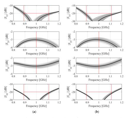
**Figure 5.** EM-driven Monte Carlo simulation of Circuit I (Figure 3a) at (**a**) the nominal design, and (**b**) the final design obtained using the proposed algorithm. MC carried out using 500 random samples. EM simulation data shown as gray curves. Black plots show the circuit responses at the nominal (**a**) and the optimized design (**b**).
