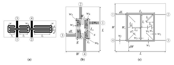
**Figure 3.** Microwave structures employed for validation of the proposed design centering algorithm: (**a**) compact rat-race coupler (Circuit I) [40], (**b**) miniaturized branch-line coupler (Circuit II) [41], (**c**) dual-band branch-line coupler (Circuit III) [42].
