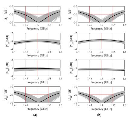
**Figure 6.** EM-driven Monte Carlo simulation of Circuit II (Figure 3b) at (**a**) the nominal design, and (**b**) the final design obtained using the proposed algorithm. MC carried out using 500 random samples. EM simulation data shown as gray curves. Black plots show the circuit responses at the nominal (**a**) and the optimized design (**b**).
