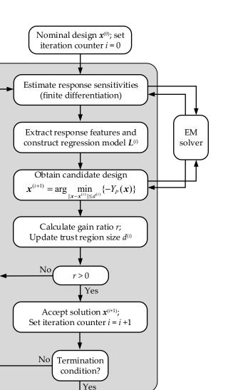
Figure 2. Operating flow of the proposed design centering algorithm.
