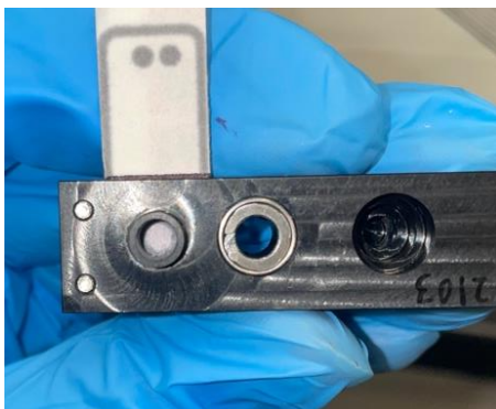
Figure 18. Photo showing a paper-based SERS substrate in the Raman spectrometer for data collection.
