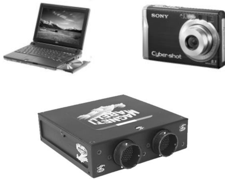
Figure 20: a general purpose machine (laptop) and two specific purpose machine: a digital camera and an engine control unit.
