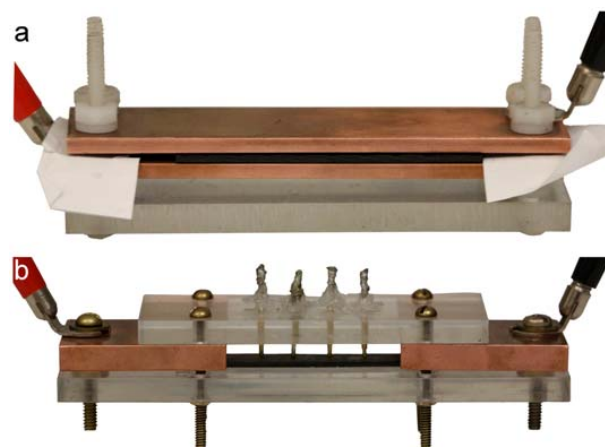
Figure 3 a sample holder used for electrical characterization of (i) nanocomposite samples in directions parallel and perpendicular to electric field and (ii) multiscale composite samples in direction parallel to electric field, i.e. through thickness (TT) of sample; b sample holder used for electrical characterization of multiscale composite samples in longitudinal direction, i.e. along length of samples (parallel to carbon fibers)
